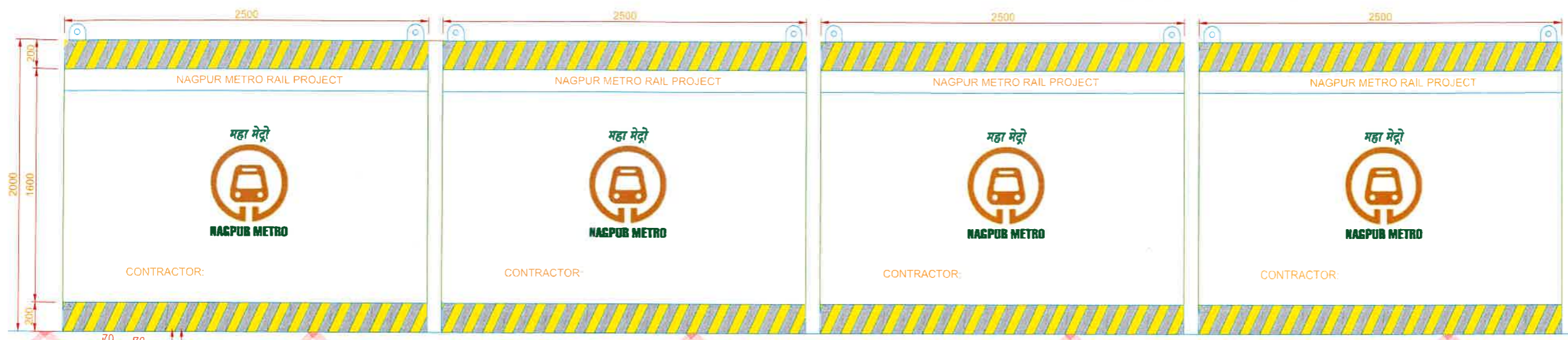
ELEVATION OF TEMPORARY BARRICADING SCALE - 1:15
